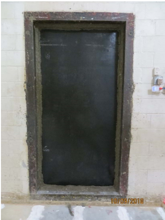
Figure 2 – Specimen mounted in test opening, as viewed from receive room
