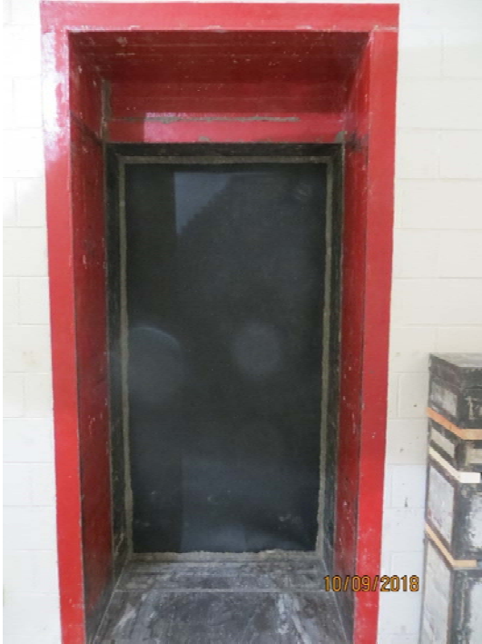
Figure 1 – Specimen mounted in test opening, as viewed from source room
