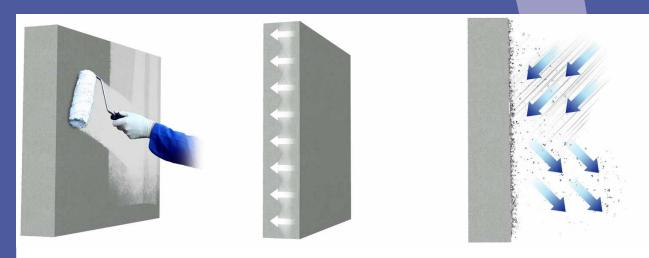
Application of InsuDry to concrete surfaces provides resistance to moisture whilst maintaining breathability of the concrete – making it an excellent choice of product for many concrete protection applications.
