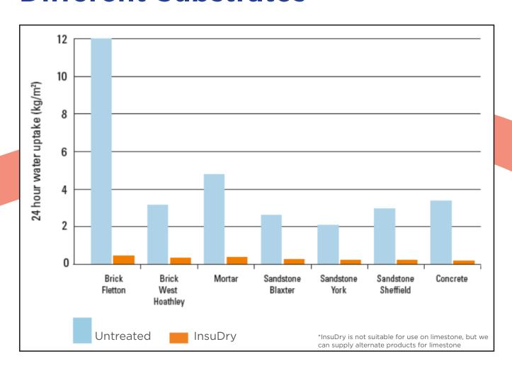
Unlike traditional liquid water-repellants, InsuDry is able to penetrate much more deeply, up to 12mm, depending on the wall type, which gives increased life expectancy and increased crack-bridging ability
